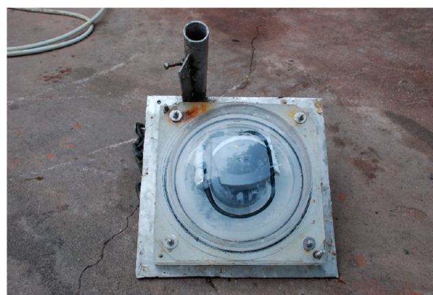
FIGURE 4. The AquaFast paint is successfully employed to protect from fouling the polycarbonate transparent hemisphere protecting the underwater camera monitoring the Cala Gadir archeological site in the Pantelleria's sea. Reproduced from with kind permission of Dr. P. Selvaggio.
